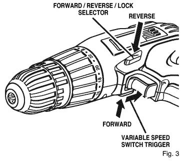
**CAUTION:** To prevent gear damage, always allow chuck to come to a complete stop before changing the direction of rotation.
